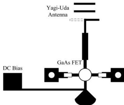
Figure 6: Layout of the active element antenna without tunable coupling network.
