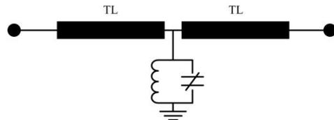
Figure 7: Schematic of tunable coupling network.
