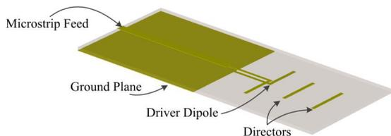
Figure 2: Geometry of the proposed antenna.
