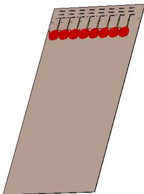
Figure 4: Geometry of the proposed antenna array for 5G mobile terminal.
