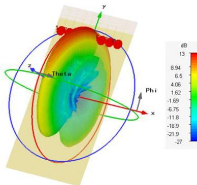
Figure 5: Simulation result of radiating pattern of the proposed antenna array for 5G mobile terminal.
