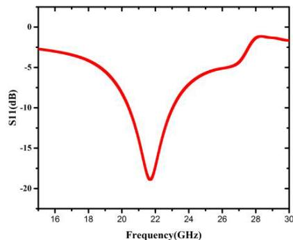
Figure 3: Simulated reflection coefficient ( $S_{11}$ ) of the proposed element antenna.
