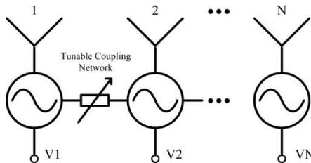
Figure 1: 1-D coupled oscillator arrays with tunable coupling network.
